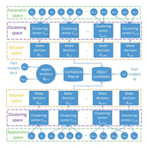
Fig. 1. Framework of the proposed clustering ensemble algorithm.  $W_i$  represents the parameter of part models in  $i^{th}$  frame.  $C_{i,j}$  denotes clustering center.  $d_{i,j}$  expresses the decisions related to  $C_{i,j}$ .
